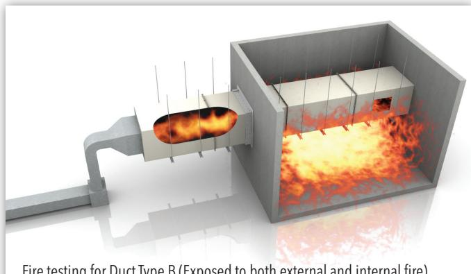
Fire testing for Duct Type B (Exposed to both external and internal fire)
